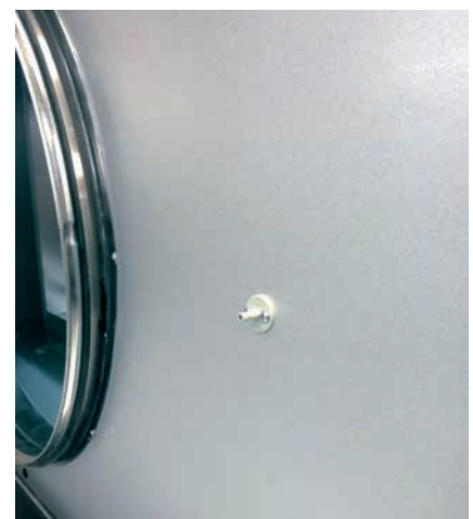
Figure 51: Tube connector for measuring duct pressure. User has to connect the attached tube to connector. The other end has to be connected to outlet air duct. The same procedure is required on inlet side. Inside CompAir, tubes must be connected to inside connectors.
