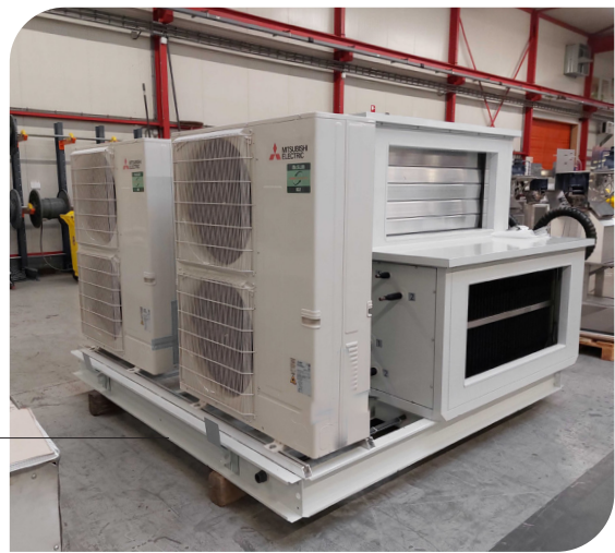
Figure 6. Basic setup with heat pumps
